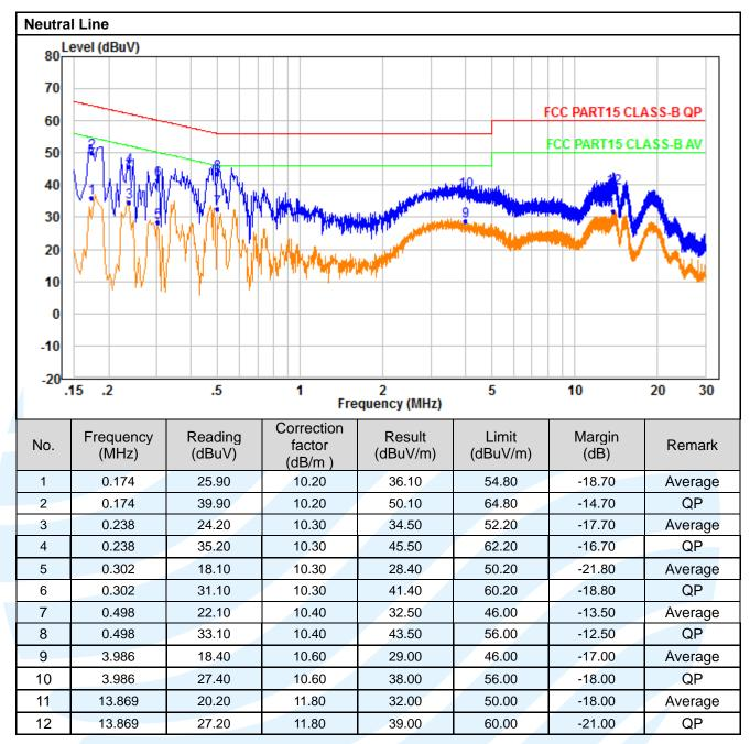
Remark: An initial pre-scan was performed on the Phase and neutral lines with peak detector. Quasi-Peak and Average measurement were performed at the frequencies with maximized peak emission were detected.
