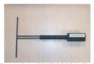
Figure 1 – Satimo COMOSAR Validation Dipole
