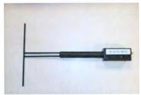
Figure 1 – Satimo COMOSAR Validation Dipole
