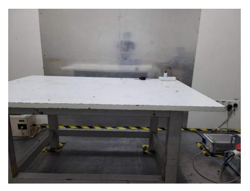
Radiated Spurious Emissions(30MHz-1GHz)
