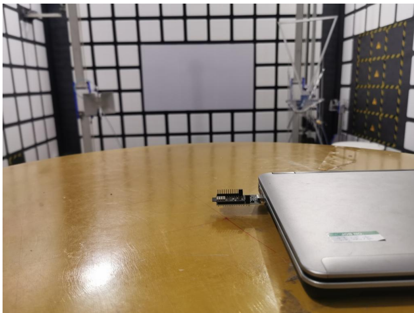
Spurious Radiated Emissions Test setup
