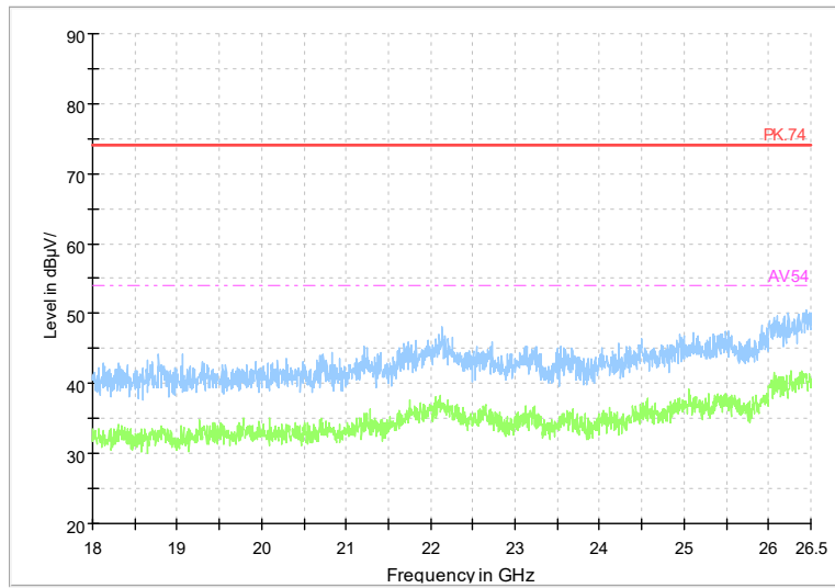
Frequency Range: 18GHz -26GHz Detector: Av mode and PK mode Modulation type: 802.11g
