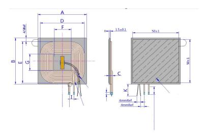
Antenna transmission frequency: 126-148KHz
