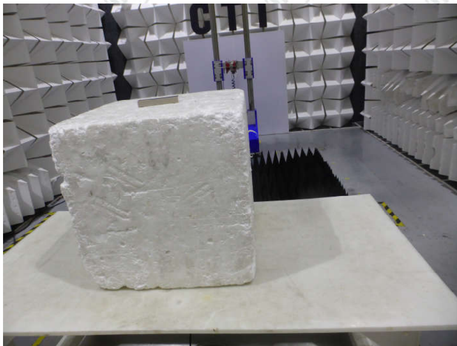
Radiated spurious emission Test Setup-3(Above 1GHz)
