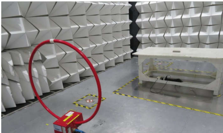
Radiated spurious emission Test Setup-1(Below 30MHz)
