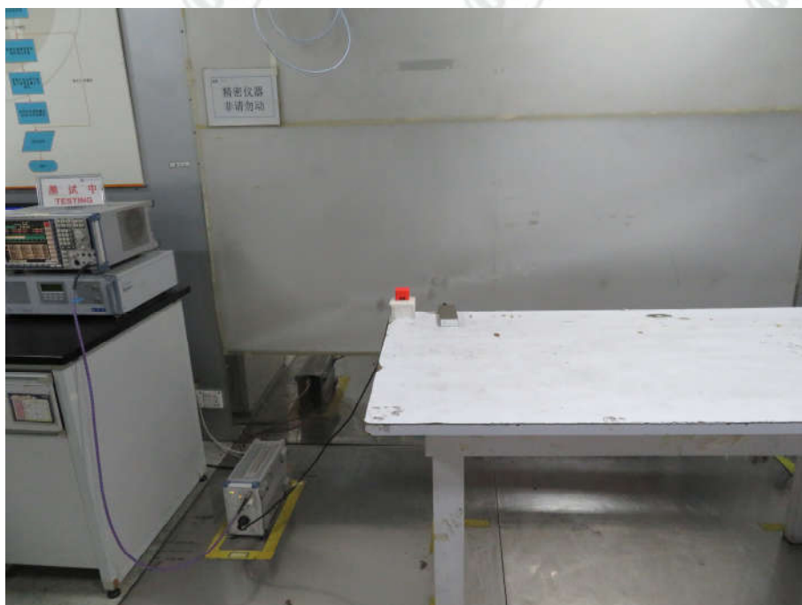
Conducted Emissions Test Setup
