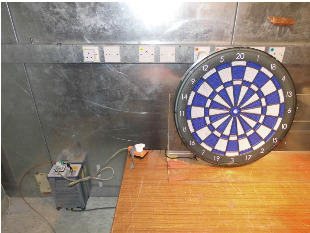
Set-up for AC Mains Conducted Emission
