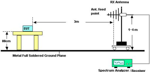
For radiated emissions from 30MHz to 1GHz
