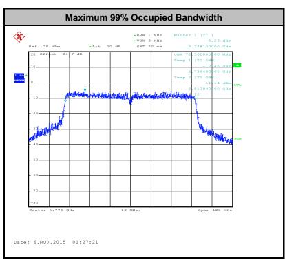
Note: The occupied channel bandwidth is maintained within the band of operation for all of the modulations.
