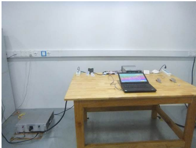
Conducted Emissions Test Setup – Front View
