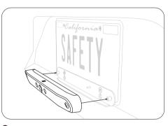
• Place your ZUS Smart Backup Camera on the mounting plate and tighten the security screws with the screwdriver.
