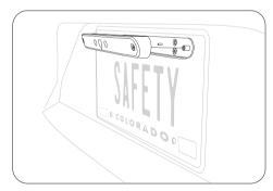
**2** Place your ZUS Smart Backup Camera on the mounting plate and tighten the security screws with the screwdriver.
