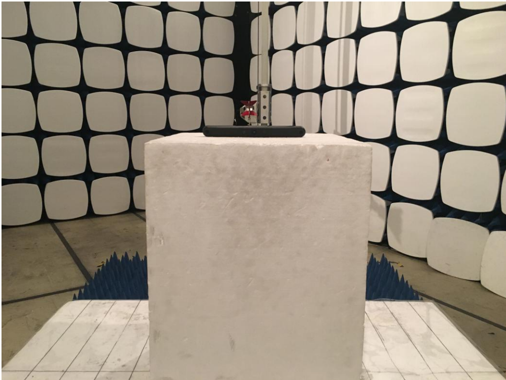
FCC RADIATED EMISSION TEST SETUP ABOVE 1GHZ
