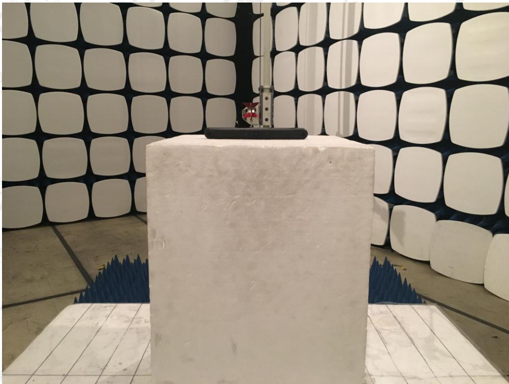
FCC RADIATED EMISSION TEST SETUP ABOVE 1GHZ
