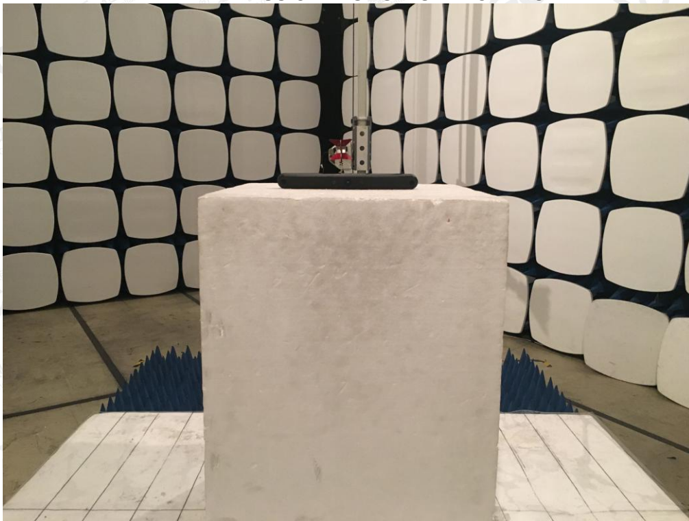
RADIATED EMISSION TEST SETUP ABOVE 1GHZ
