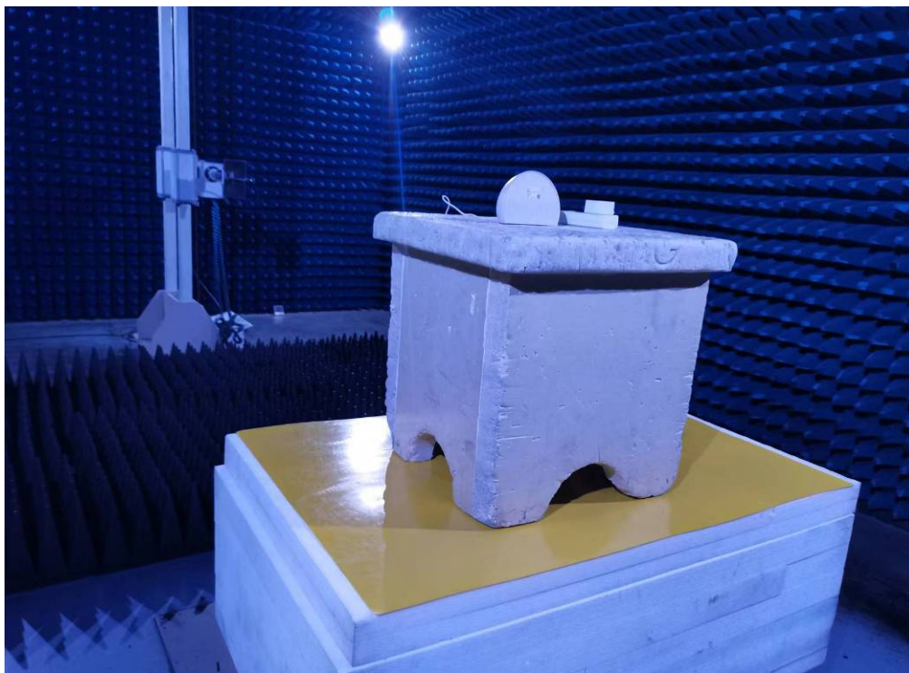
Photo of Radiated Emission Measurement (Above 1G)
