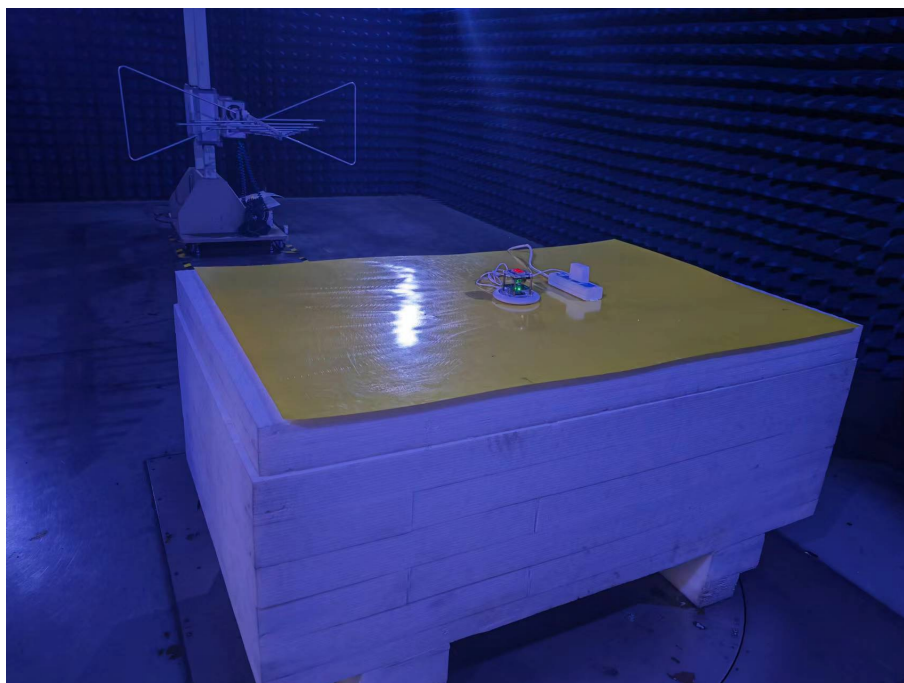
Photo of Radiated Emission Measurement (30MHz-1GHz)
