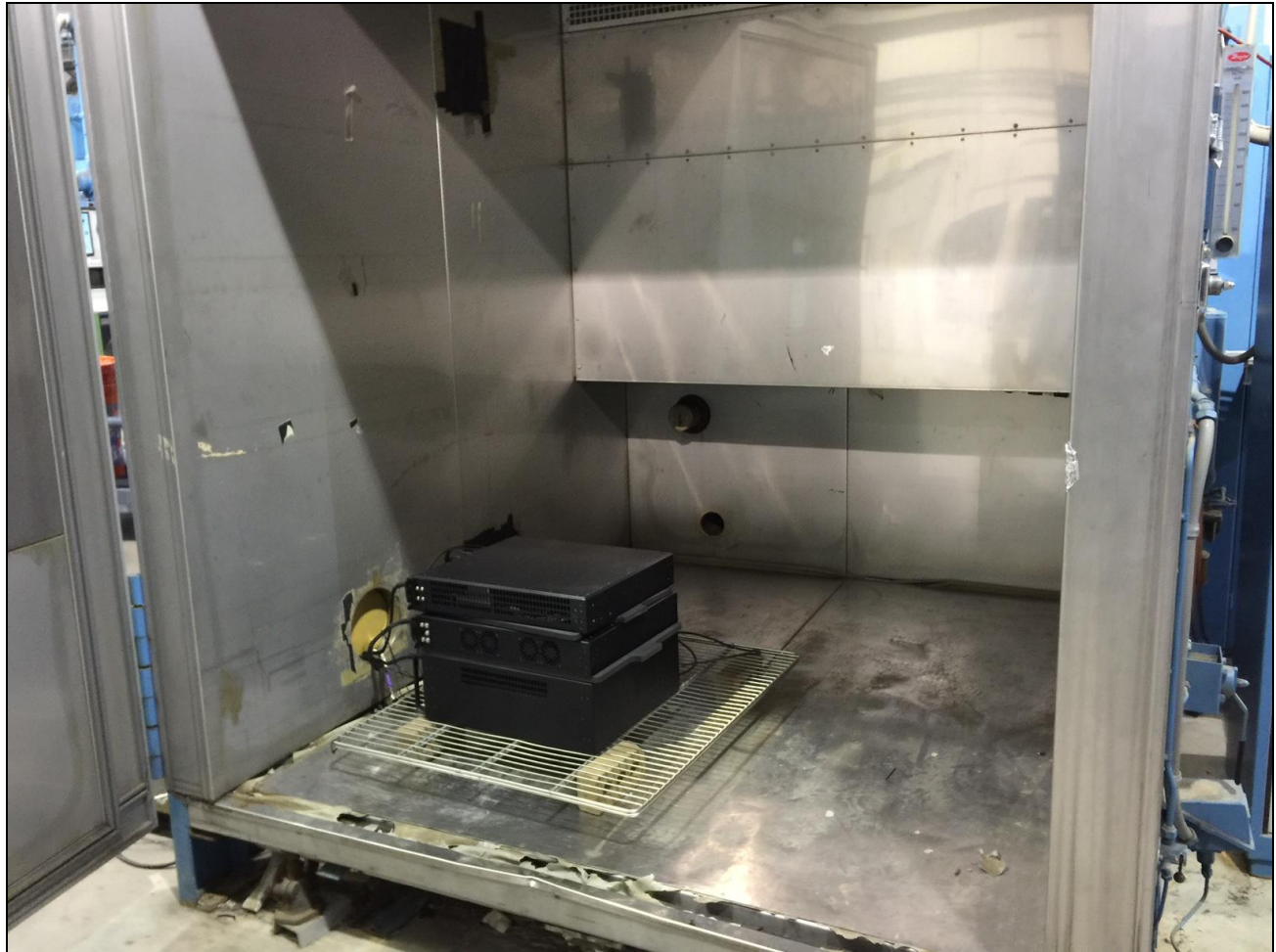
Photograph 2. Frequency Stability, Test Setup
