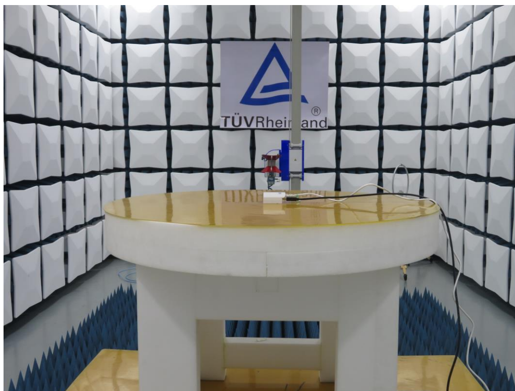
Photograph 2: Set-up for Radiated Spurious Emission, Above 1GHz
