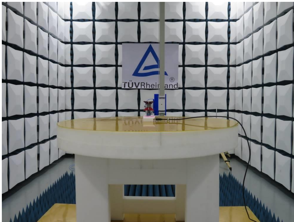
Photograph 2: Set-up for Radiated Spurious Emission, Above 1GHz
