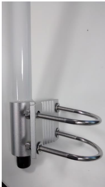
Mount the U bolts on the antenna
