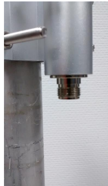
Remove the cap on the N connector of the antenna
