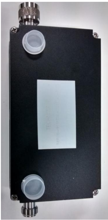
Remove caps on both N connectors
