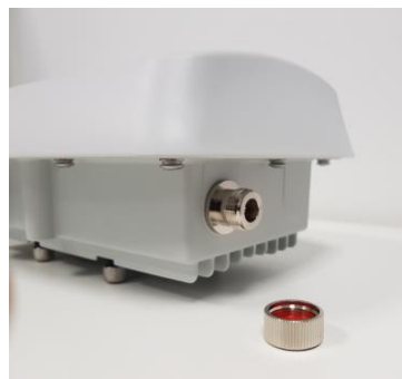
Unscrew RF switch cap
