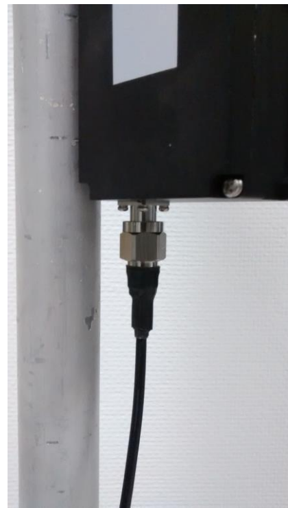
Screw the coaxial cable onto the N connector of the cavity filter
