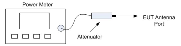
The measure is realized in conducted mode with a calibrated gated RF average reading power meter.
