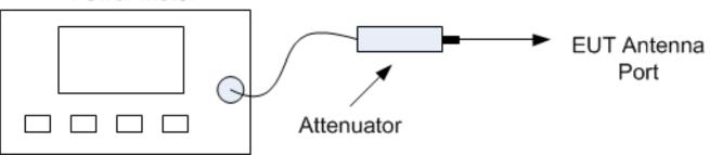
The measure is realized in conducted mode with an analyser.
