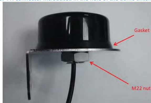
Figure 108 : Antenna installed on the dome antenna bracket
