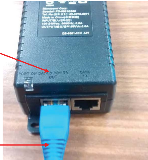
Figure 157 : Ethernet connection on PoE injector side
