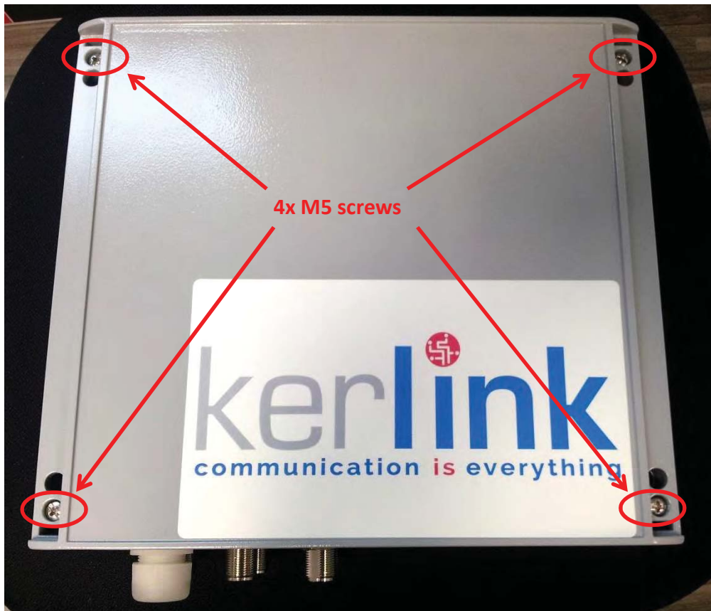
Figure 95: Wirnet iBTS – 4x M5 screws
