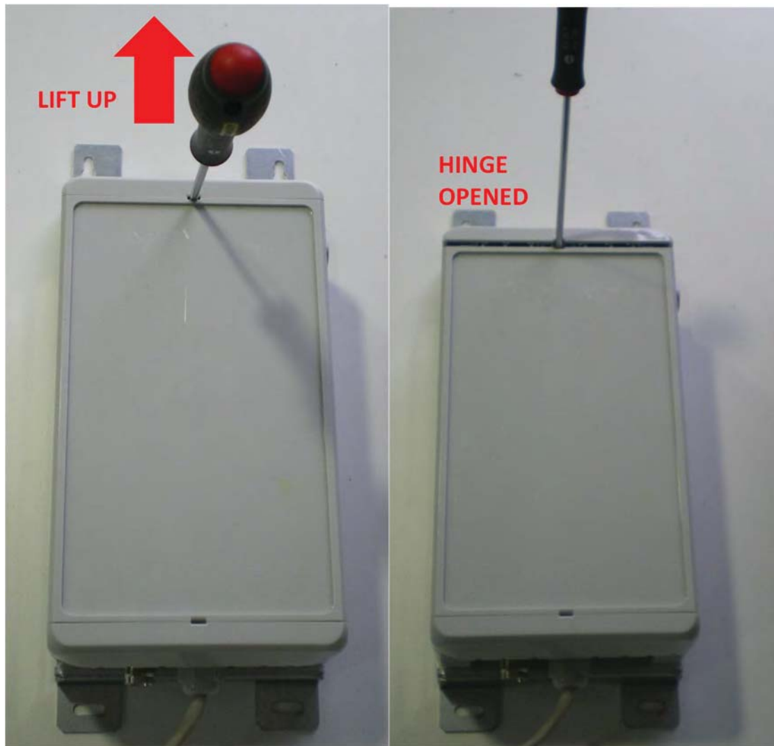
Figure 97 : Opening of the compact enclosure with screwdriver
