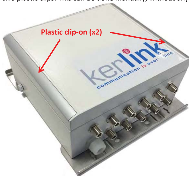
Figure 94: Wirnet iBTS – plastic clips on the lid
