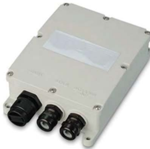
Figure 42 : Outdoor 30W AC/DC POE injector
