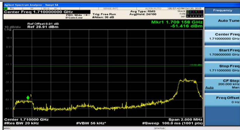
(Channel Bandwidth:15 MHz)_LCH_16QAM_37RB#0
