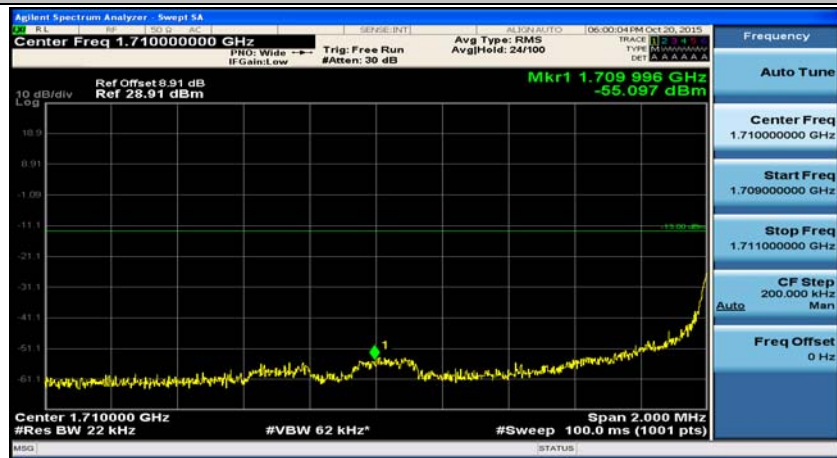
(Channel Bandwidth:20 MHz)_LCH_QPSK_50RB#0
