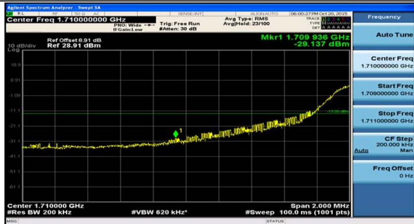
(Channel Bandwidth:20 MHz)_LCH_QPSK_50RB#25
