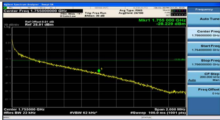
(Channel Bandwidth:20 MHz)_HCH_16QAM_50RB#0
