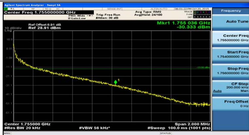
(Channel Bandwidth:20 MHz)_HCH_QPSK_50RB#0
