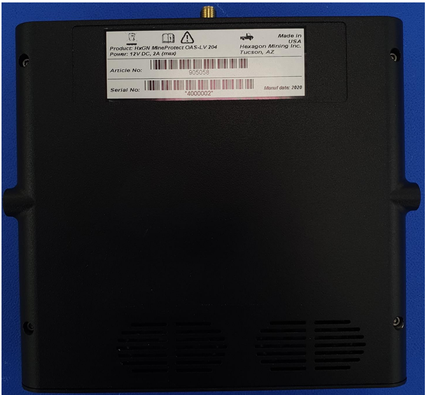
Figure 7 OAS-LV 204 Bottom View with FCC ID, Serial Number and Article Number Label
