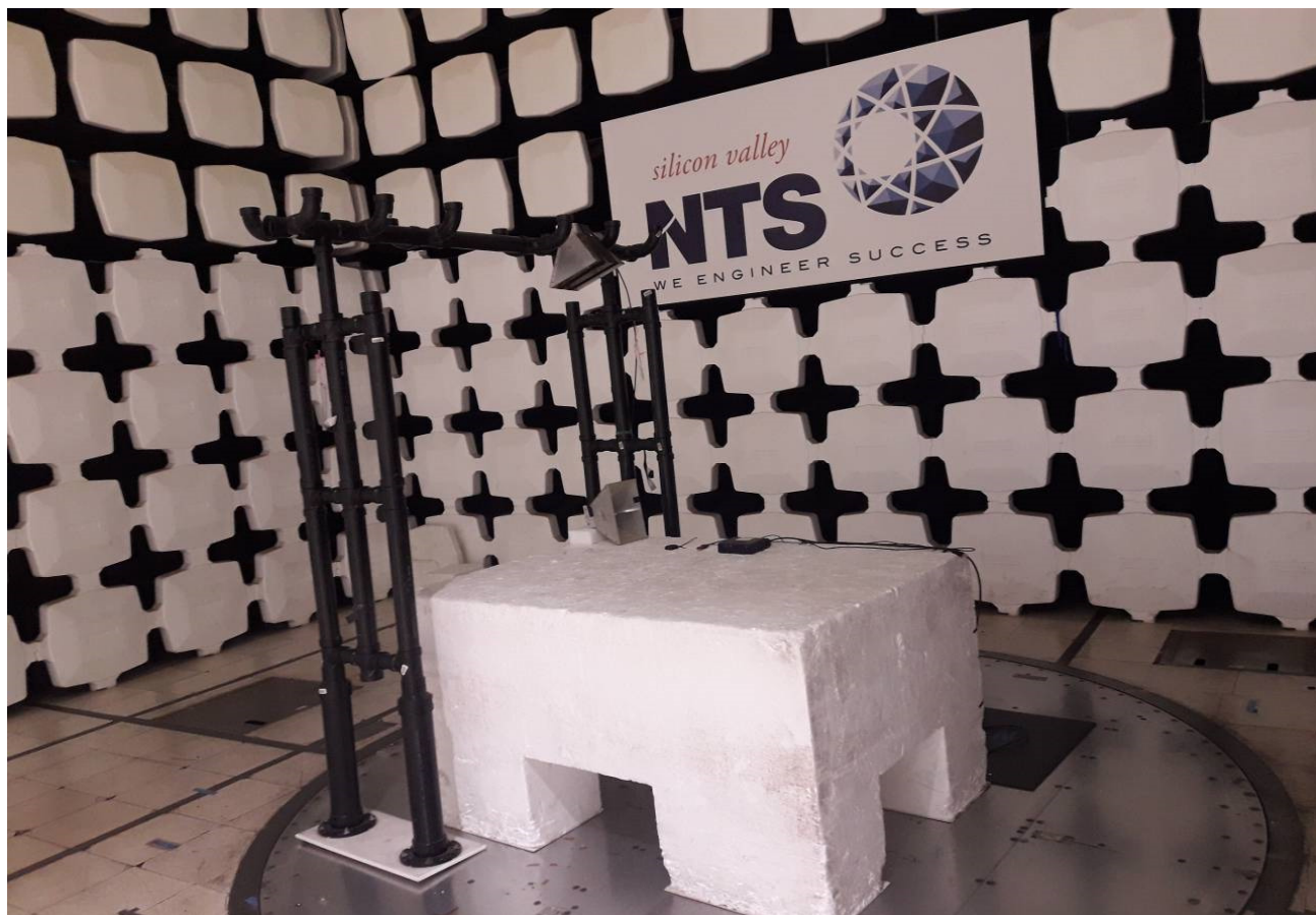
Test Configuration Photograph #1 (Radiated Emissions)
