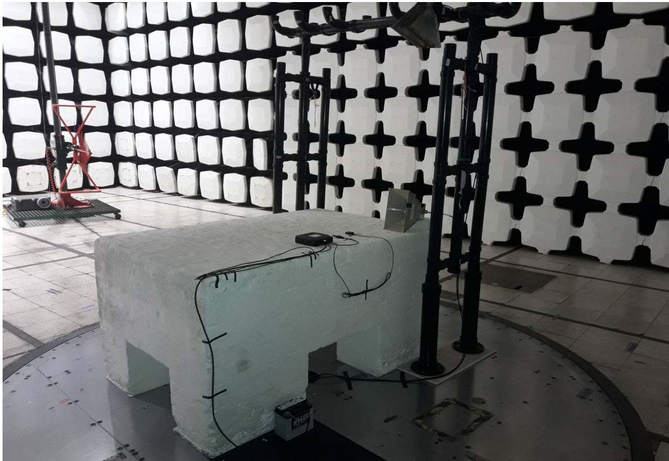
Test Configuration Photograph #2 (Radiated Emissions)
