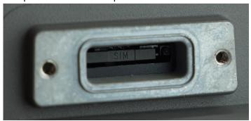
4. Place data SIM card into SIM card holder with the chip facing up
