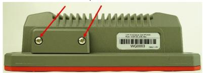
3. Use a pointed instrument to press the release mechanism.
