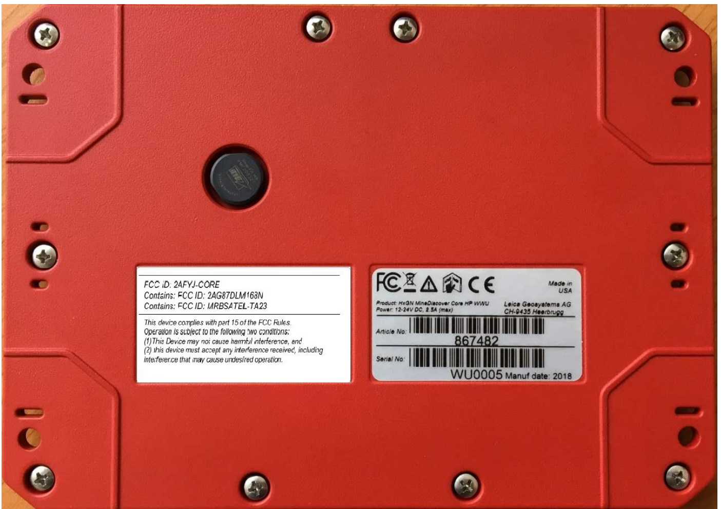
Figure 4 CoreHP Bottom View with FCC ID, Serial Number, and Article Number Labels
