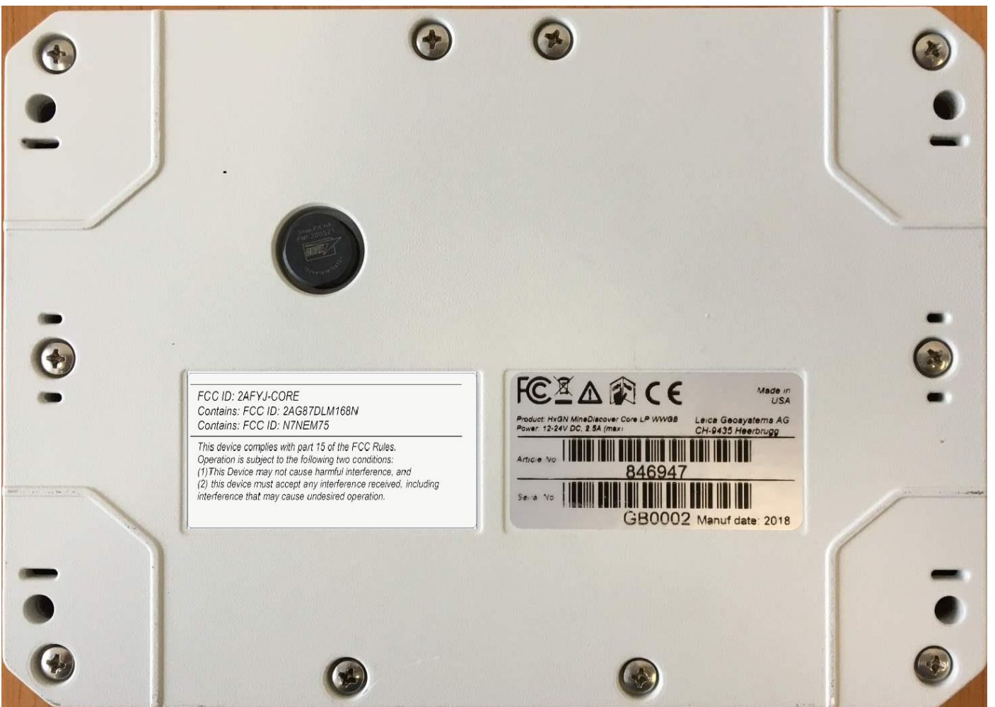
Figure 9 CoreLP Bottom view with FCC ID, Article Number, and Serial Number, Labels
