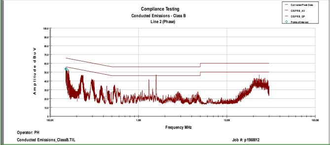
The signals at 1.30 and 1.57 MHz are ambient test signals and not part of the EUT.
