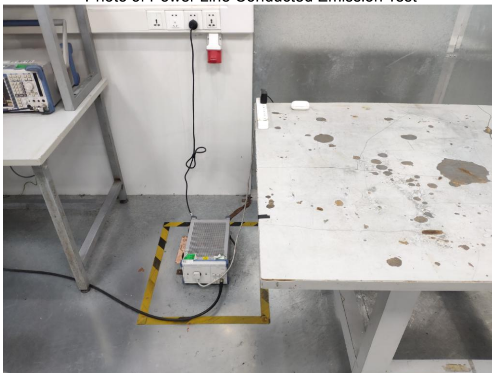
FCC ID: 2AFYE-J513A Photo of Power Line Conducted Emission Test
