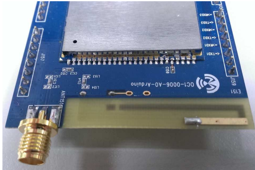
Figure11-1.Reversed SMA connector to connect dipole antenna
