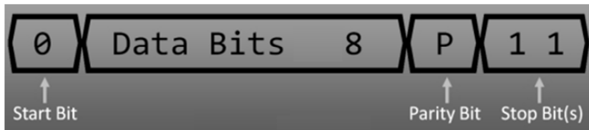
Figure7. UART Data Format
