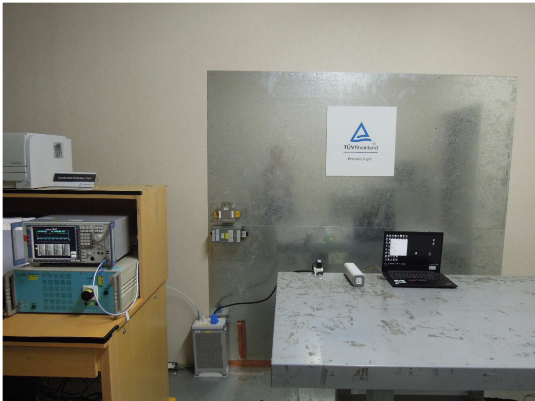
Photograph 6: Set-up for for AC Mains (Front)
