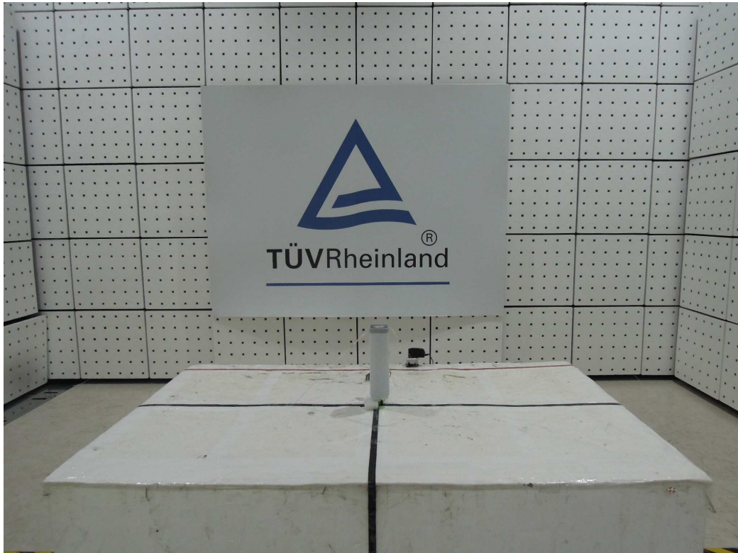
Photograph 2: Set-up for Spurious Emissions (Back View 1)
