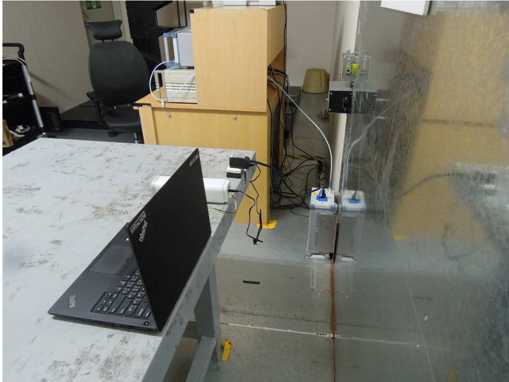
Photograph 6: Set-up for for AC Mains (Front)
