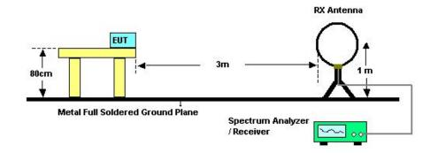
For Radiated Emissions: 30MHz~1GHz
