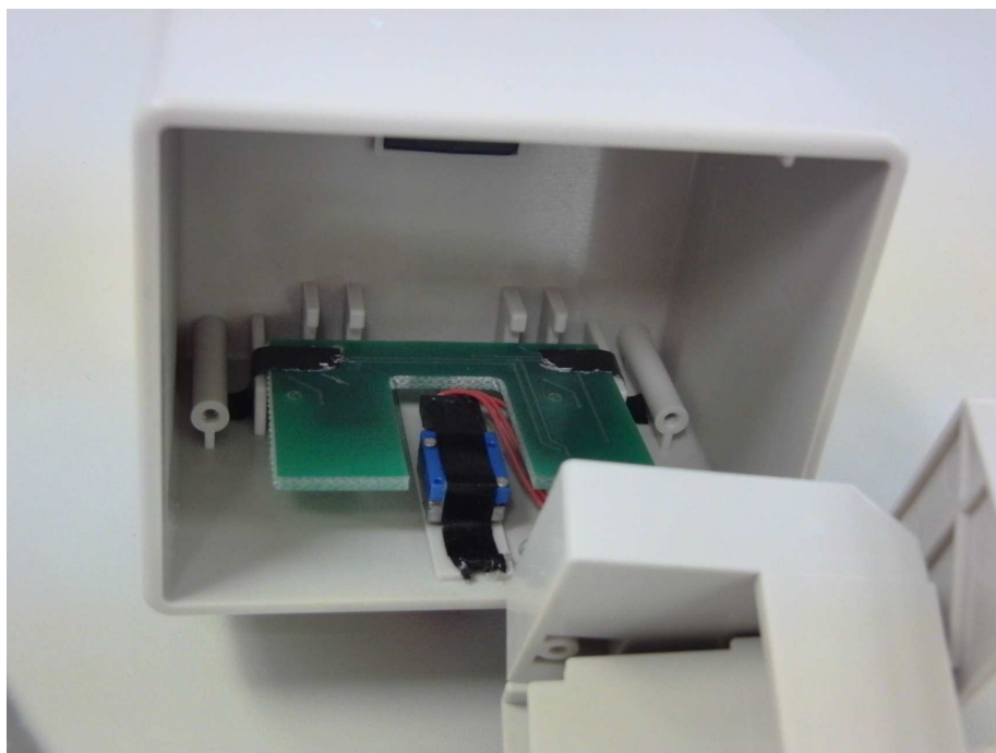
LED board (eyes) and potentiometer (nose)
