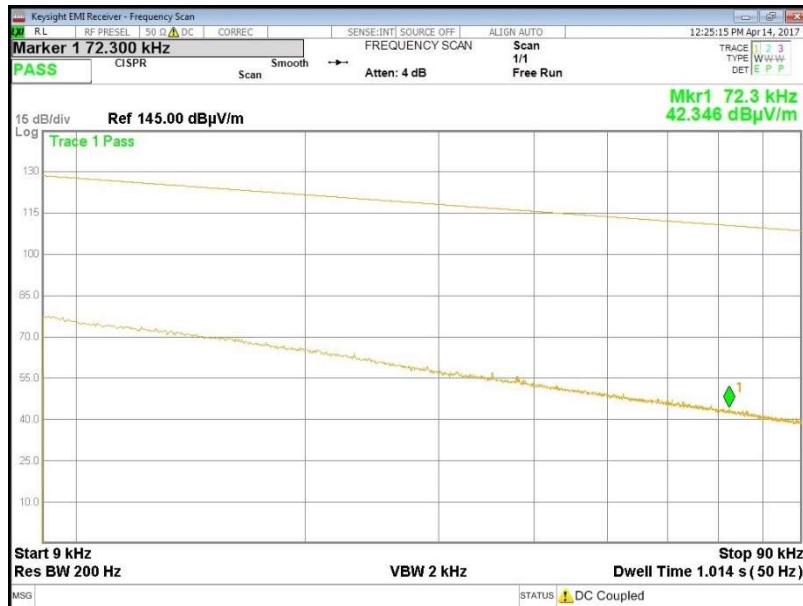
Fig. 3 - Plot referred to the Loop Antenna in Orthogonal polarization in the range 9-90 kHz
