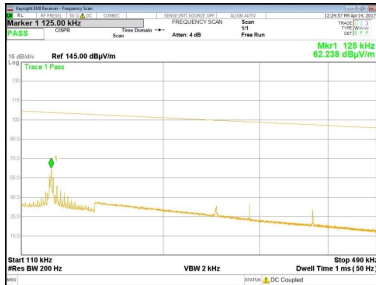
Fig. 5 - Plot referred to the Loop Antenna in Parallel polarization in the range 110-490 kHz
