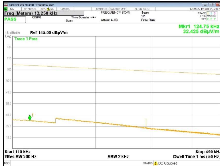
Fig. 4 - Plot referred to the Loop Antenna in Orthogonal polarization in the range 110-490 kHz
