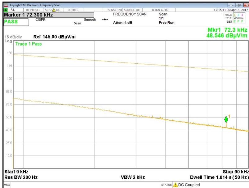
Fig. 2 - Plot referred to the Loop Antenna in Parallel polarization in the range 9-90 kHz
