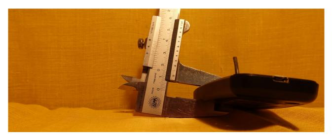
We taking into account that **the housing grantee a minimum distance of 7.5 mm** as separation between the Bluetooth antenna inside the device and the closest hand surface in contact with the external device in the correlated point of the Bluetooth antenna. Accordingly with this our measurements and the SILICON Lab evaluation about the SAR, we can confirm on the HC1000 that the SAR measurement can be excluded.
