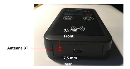
Accordingly with the Bluegiga report we can confirm that the Bluetooth transmission operates in the BT121 module for 300,1ms in a period of 31,6 seconds, we can treat the object of the par.6.3 of the KDB 447489 D01 "General RF Exposure Guidance" v06 and considering for the EZ-sensor PAD, as the same of the HC1000, as Low transmission duty factor device.
