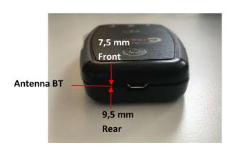
Accordingly with the Bluegiga report we can confirm that the Bluetooth transmission operates in the BT121 module for 300,1ms in a period of 31,6 seconds, we can treat the object of the par.6.3 of the KDB 447489 D01 "General RF Exposure Guidance" v06 and considering the HC1000 as Low transmission duty factor device.
