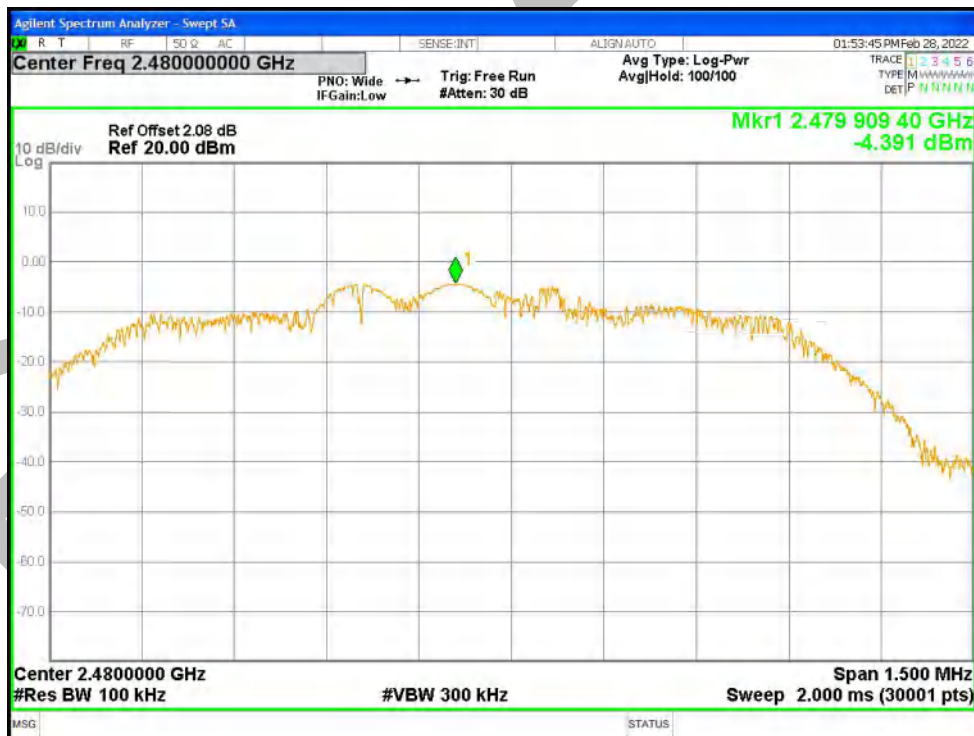
Tx. Spurious NVNT 2-DH1 2480MHz Ant1 Emission
