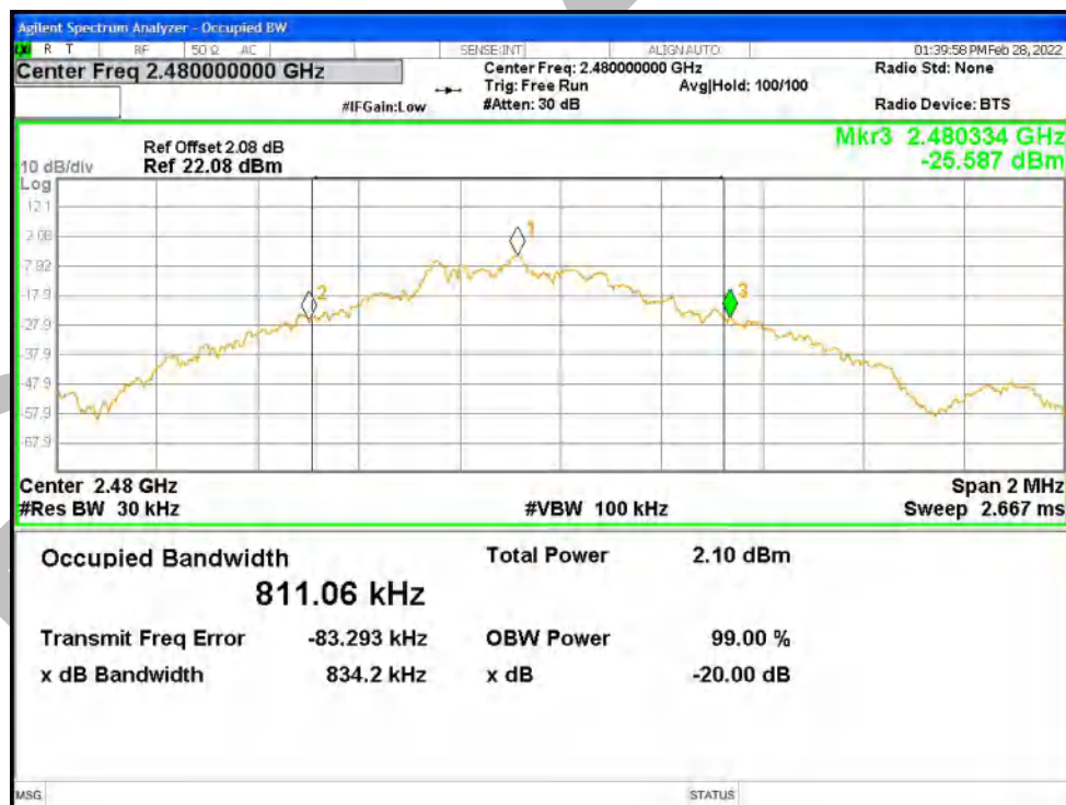
-20dB Bandwidth NVNT 2-DH1 2402MHz Ant1
