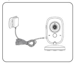
Connect the camera power to the transformer supplied. The blue LED turns on to indicate that it is running.
