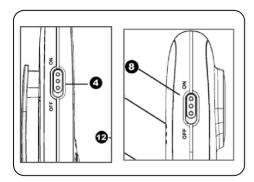
Push the power key up to turn the monitor and camera on
