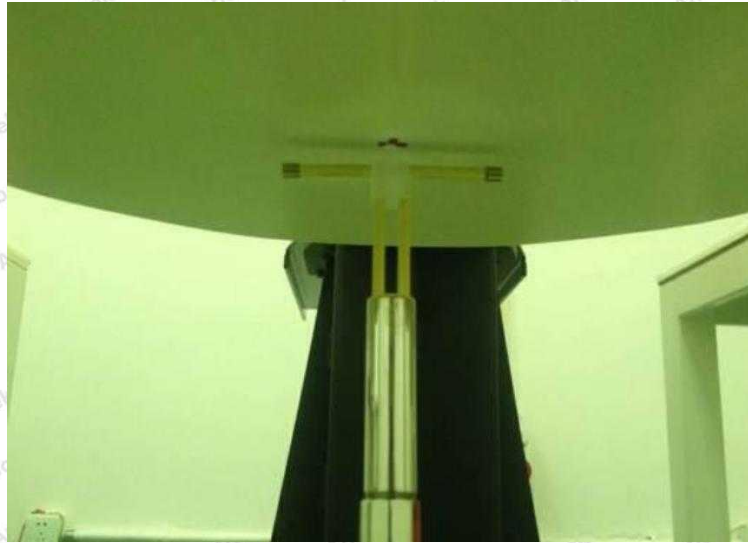
Photo of Dipole Setup
