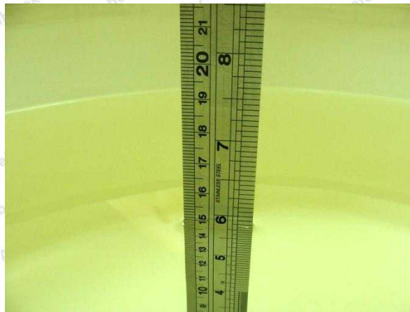
Photo of Liquid Height for Body SAR
