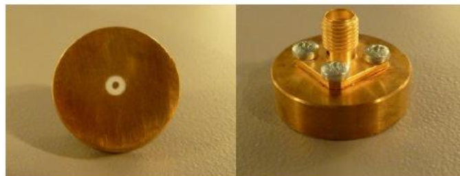
Figure 1 – MVG LIMESAR Dielectric Probe
