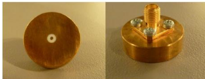
Figure 1 – MVG LIMESAR Dielectric Probe
