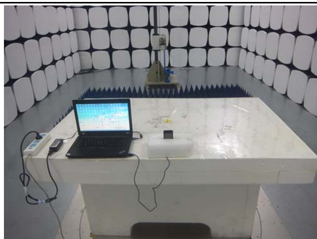
Radiated Spurious Emissions Test Setup Above 1GHz
