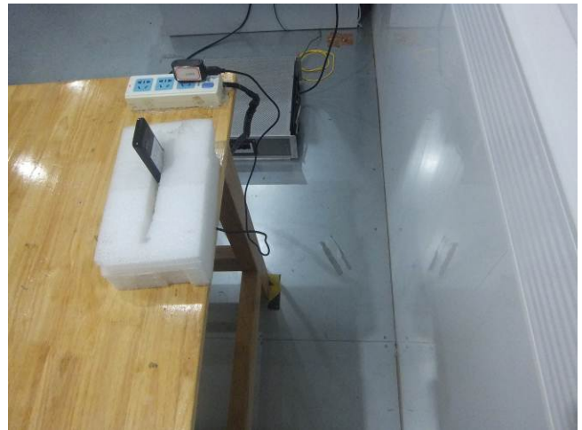
Conducted Emissions Test Setup Side View
