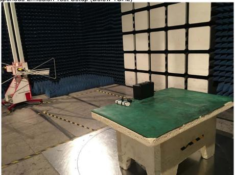
Spurious Emission Test Setup (Below 1GHz)
