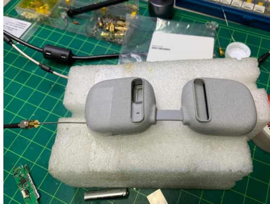
Figures 2-1.1 Measurement Setup of SOLUM BLE MASK device.
