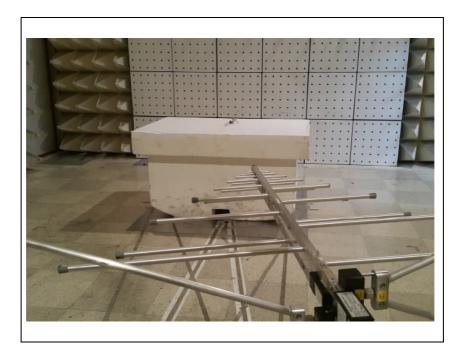
B. Photo of Radiated Spurious Emission Test (Above 1 🕮)
