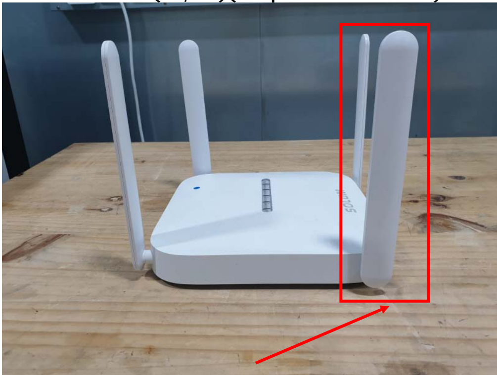
Antenna 2(TX, RX)(Freq : 2402-2480 MHz)
