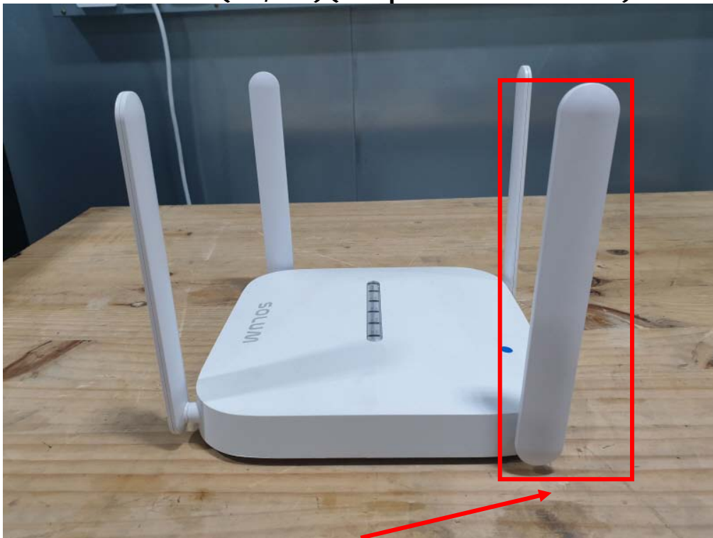
Antenna 4(TX, RX) (Freq : 902.4-927.6 MHz)
