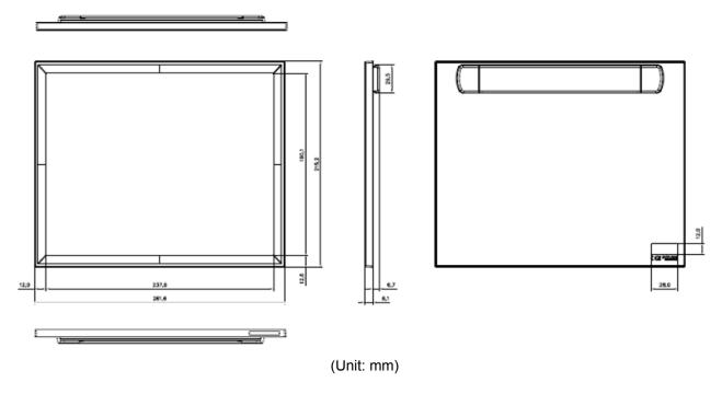
Figure 7. 12.2" Mechanical Dimension
