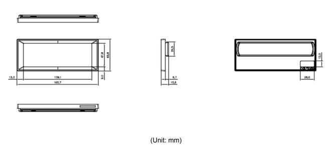
Figure 5. 5.85"Freezer Mechanical Dimension
