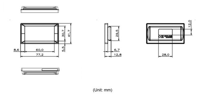
Figure 3. 2.6" Mechanical Dimension
