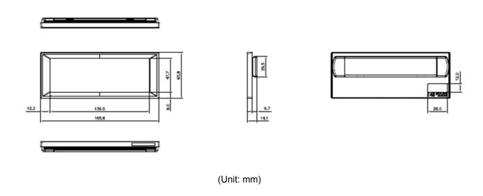
Figure 4. 5.85" Mechanical Dimension
