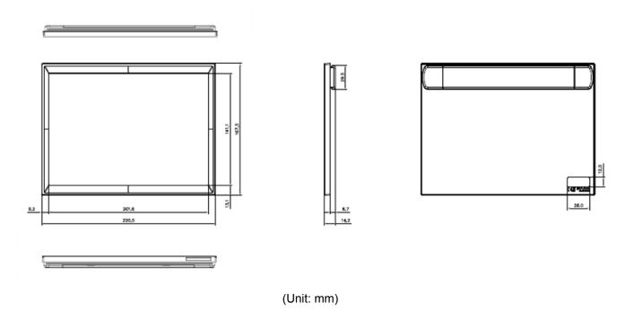
Figure 6. 9.7" Mechanical Dimension
