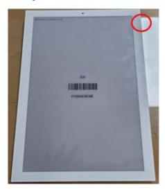
Press the button for 3 seconds and then ESL screen will be off.
